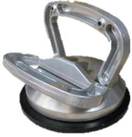
Before fixing the posts the circular covers for the post fixing holes have to be removed using the sucker in STORE 2. Open the handles up, as shown here, press the sucker onto the cover then bring the handles together. It should then be possible to lift the cover.
