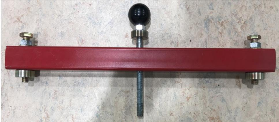
The brass rings at either end will sit on the two lugs on the base of the posts. The central bolt goes into the floor:
